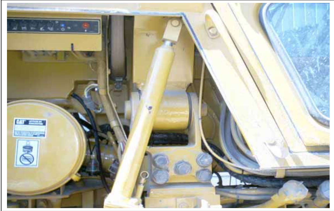
Hose routing to opening in bottom of cab. Run so that the cab can be tilted up.
